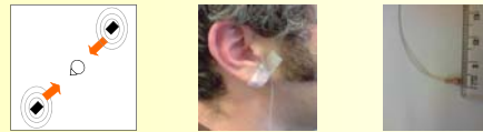
Figure 2. In the canal microphone recordings, test booth set-up (left), microphone positioned in ear canal (centre), the microphone used for recordings (right).
