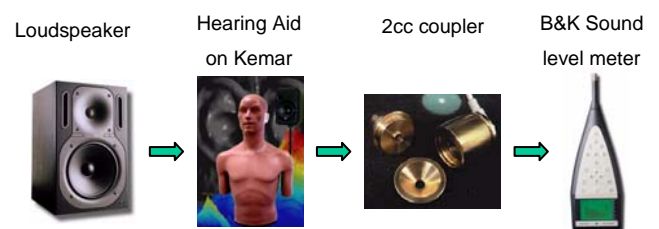
Figure 1. Setup for acoustic measurement of hearing aid output levels.
